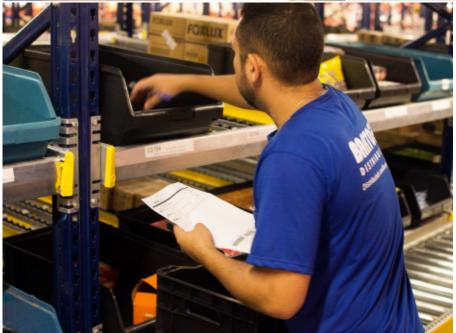
Live picking shelves run between the blocks of live racking. They comprise three roller platforms and are set on a slight incline so that boxes slide through gravity. The advantage of these solutions is that stock is always available, meaning pick tasks can be carried out.
