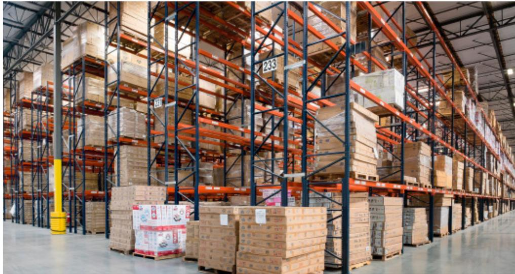
Delta Children's new warehouse features 47 aisles of pallet racking aisles that can store 30,606 pallets in a 26,938 m<sup>2</sup> area
