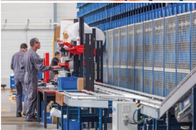
The new Grégoire-Besson logistics centre, a French farm technology equipment company, consists of an automated warehouse for boxes, pallet racking and cantilever racking by Mecalux. The combination of these three storage systems lets merchandise be organised according to their characteristics and demand, streamlining order picking tremendously.
