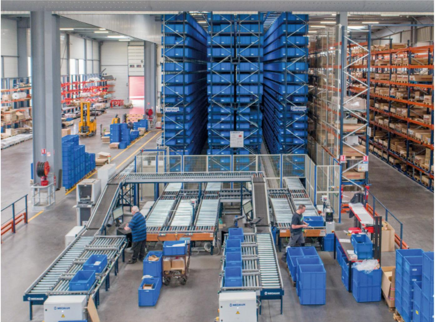
The warehouse is composed of two aisles with double-deep racking on both sides that measure 47 m long, 9 m high and have 17 shelves.
