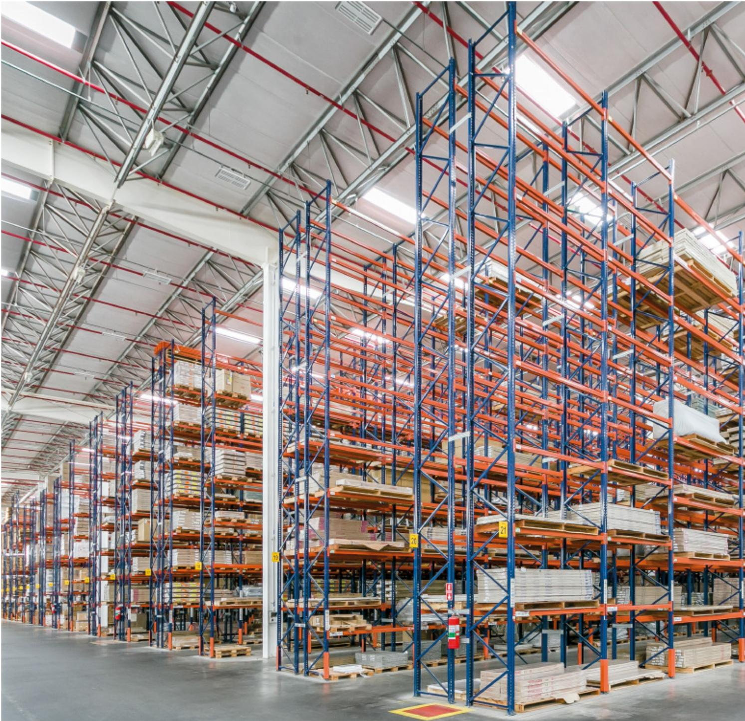
**Mecalux has set up pallet racking in the warehouse Magazine Luiza, an electronics company, owns and operates in the Brazilian city of Guarulhos. With this system, the company has attained a capacity to store more than 15,300 pallets.**
