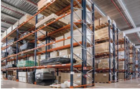
or six shelving levels. One of its main advantages is the adaptability to any type of load, weight and volume variable. Different product types are slotted on the shelves: from large-sized pallets to foldable chairs. Plus, the direct access feature of the system
