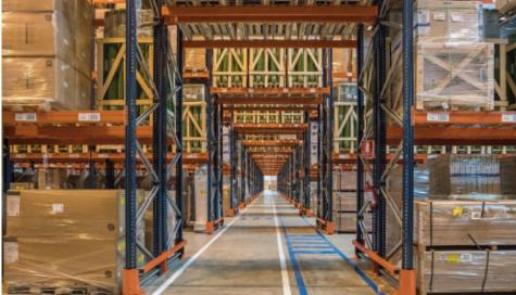
Operators work via zones and are assigned to a few working aisles. They use forklifts to insert and extract pallets from their corresponding locations.
