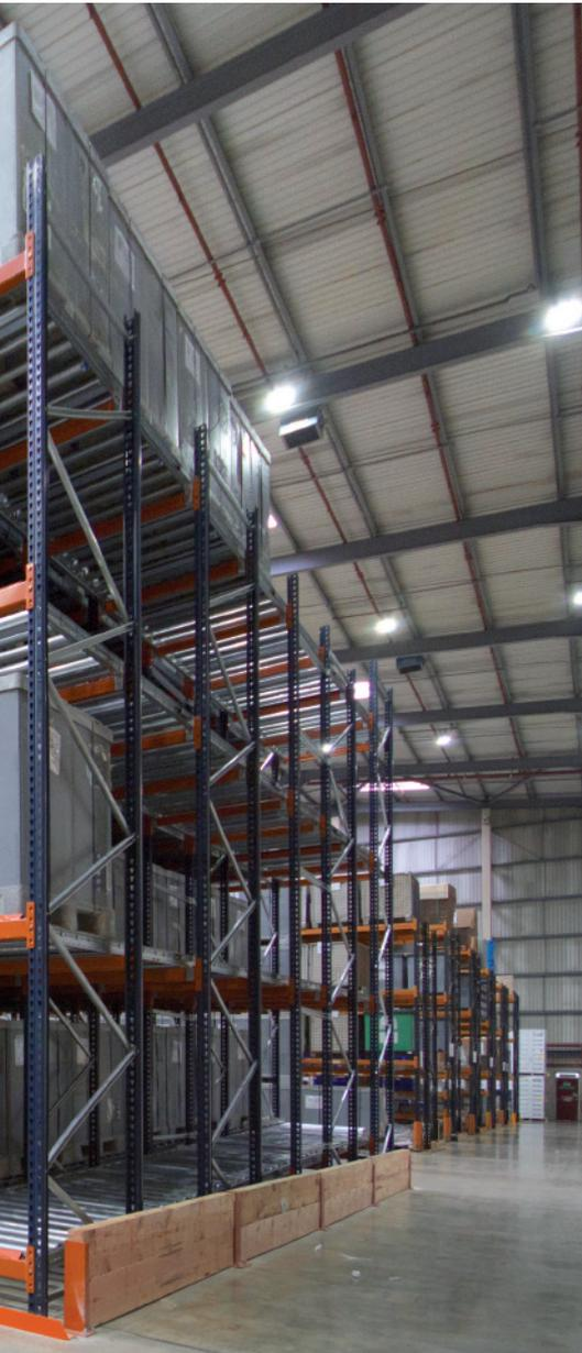
The racks are composed of roller channels with a slight incline that allows gravity flow of the pallets
