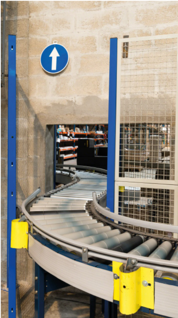
The hinged conveyor section can open so that operators may cross from one area to another
