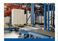
1. The shuttle picks up a pallet from the inbound conveyor in front of the racking.
