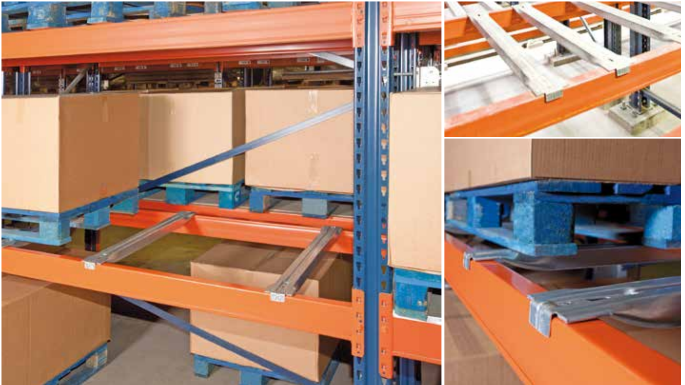
Close-up of a galvanized pallet support bar
