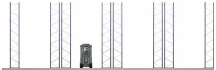
The most common pallet racking system , comprising single-access racks fitted to the walls and double-access (back-to-back) racks in the middle
