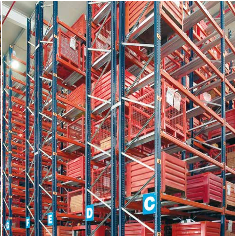
Selective pallet racking system with metal containers
