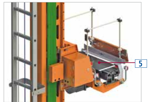
Cradle or mobile lifting frame (5)
