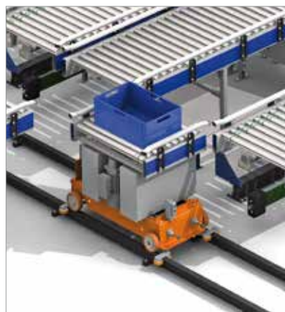
Details of a shuttle (1).
