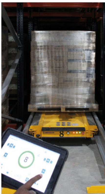
An aisle lines each side of each block of racks. The goods can be managed as per the FIFO principle (i.e., insert the pallets through one aisle and extract them from the opposite aisle) or the LIFO method (insert and extract pallets from the same aisle), depending on Tamer's logistical requirements.
