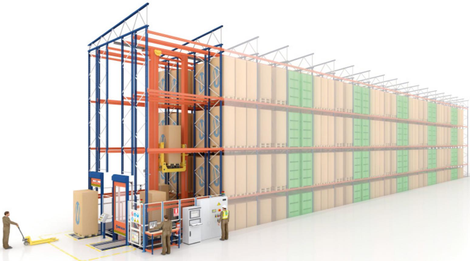
The racking, divided into four levels, has been personalised to be able to accommodate three different unit loads: 1,200 x 1,200 mm plastic containers and pallets measuring 800 x 1,200 mm and 1,000 x 1,200 mm. In the case of plastic containers, each location can store up to four containers stacked one on top of the other.
