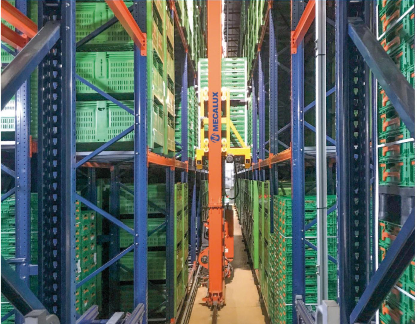
**Kiwi Greensun, the Iberian Peninsula's largest producer of kiwis, has overhauled its fruit ripening room in Salvador de Briteiros, Portugal, with the construction of an automated clad-rack warehouse by Mecalux managed by Easy WMS. With this installation, the company has its sights set on raising production to 12,000 t of kiwi fruit a year. One of the advantages of this warehouse with fully automated operations is the accurate control of products stored at refrigerated temperature.**
