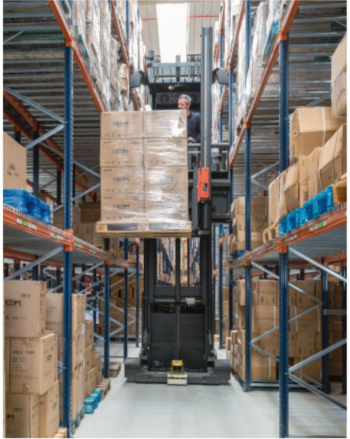
ing the products they need. To meet all of Elektro3's requirements, Mecalux has installed pallet racking with narrow aisles for three reasons: its adaptability to any type of load, weight and volume; the direct access it offers to the products (facilitating goods handling and order picking); and its optimisation of space.
