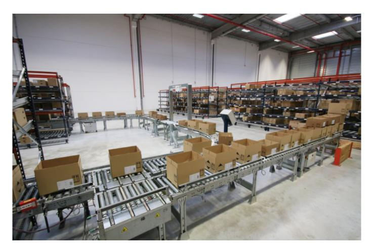
Although the continuous circuit is "U" shaped, boxes that need medium and low turnover products are diverted to an accumulation conveyor, awaiting the operator assigned to this area to start preparing those SKUs.
