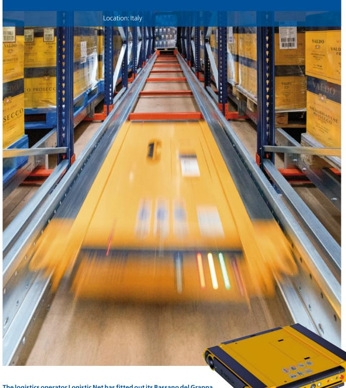
The logistics operator Logistic Net has fitted out its Bassano del Grappa (Italy) warehouse with high-density racking run by four Mecalux Pallet Shuttles, tasked with moving goods inside the storage channels. With this solution, this integrated 3PL specialist can store more than 3,000 pallets and control them via a control tablet.
