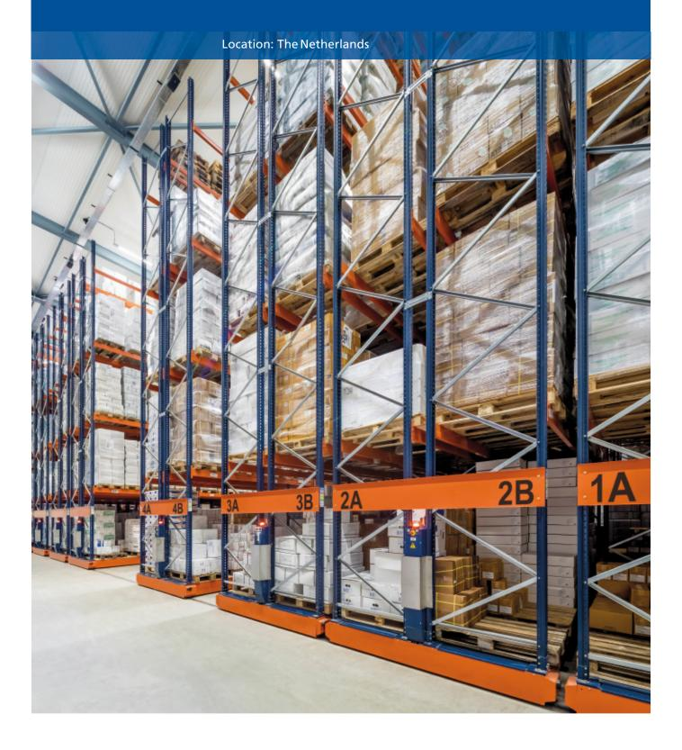
The Dutch fishing company Mooijer-Volendam B.V. has equipped one of its frozen-storage chambers with Movirack mobile pallet racking from Mecalux. This solution makes optimal use of all the warehouse's surface area and provides storage capacity for 4,349 pallets.
