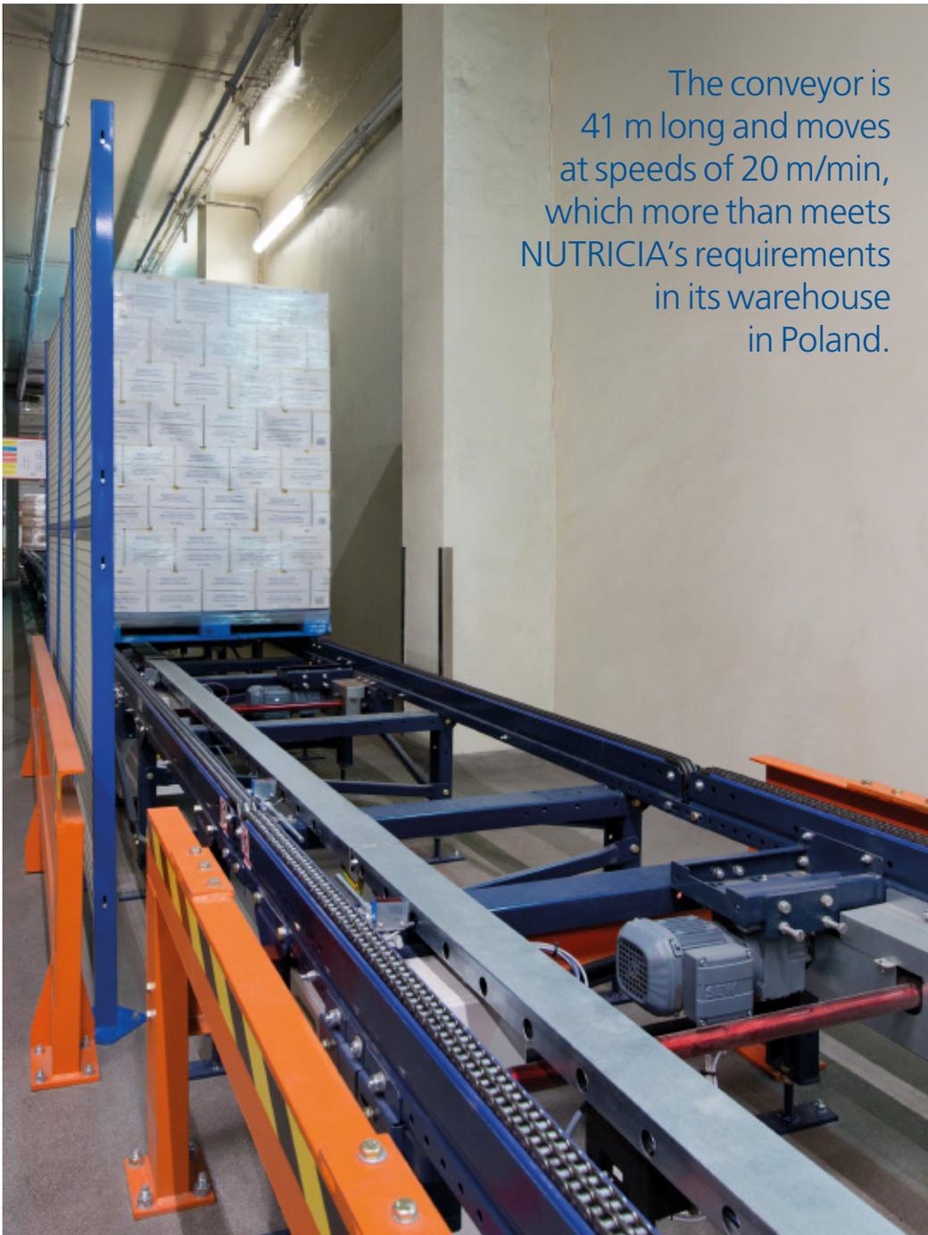
The conveyor is 41 m long and moves at speeds of 20 m/min, which more than meets NUTRICIA's requirements in its warehouse in Poland.
