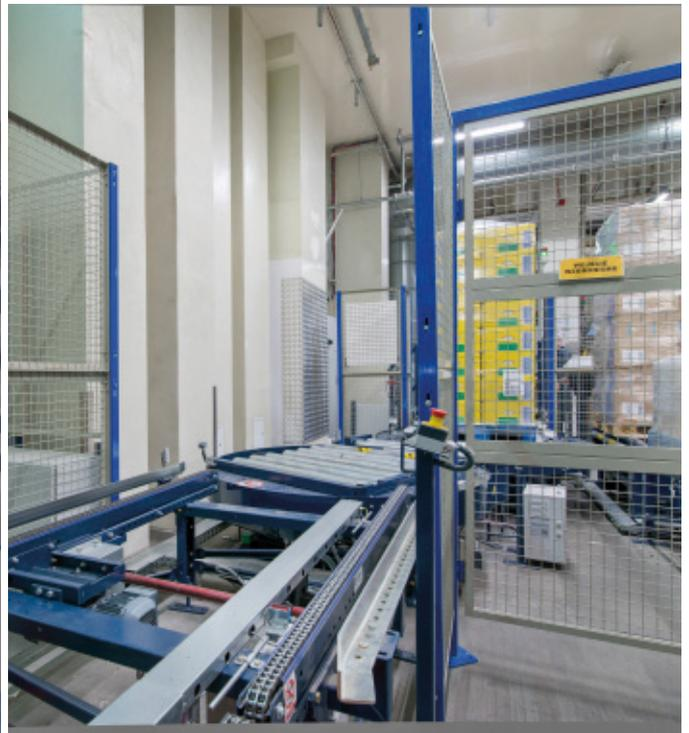
Mecalux has installed a conveyor tasked with moving goods directly from the NUTRICIA production centre to the warehouse's dispatch zone. This conveyor system cuts out the use of traditional handling equipment to shift goods between two points. By lessening manual load handling, this increments general safety in the installation significantly.
