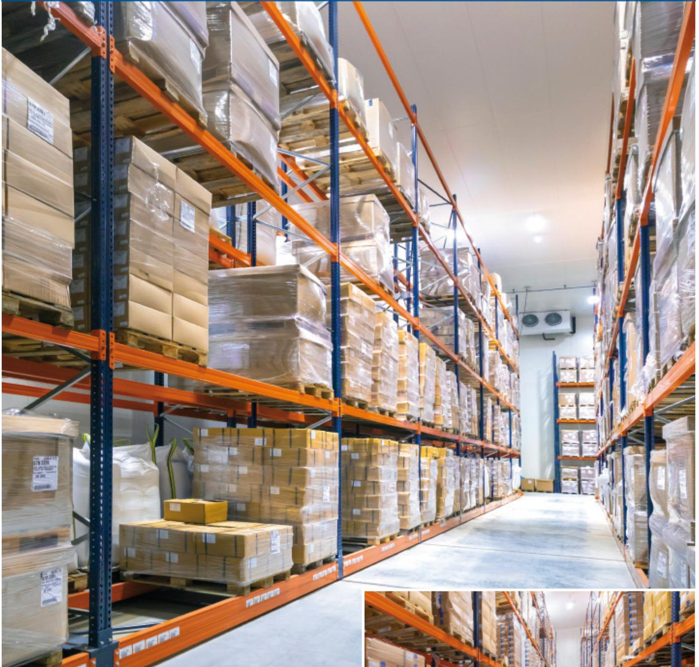
The Sabarot frozen-storage chamber in Chaspuzac (France) has 9.5 m high Movirack mobile pallet racks by Mecalux. This solution leverages all available surface area to achieve higher storage capacity and reduces power consumption to chill the installation. In total, 1,816 pallets can be deposited here filled with finished products.
