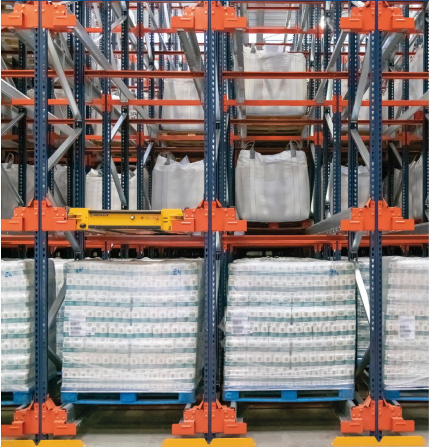
Zuidnatie, a well-known logistics specialist in Antwerp, has reworked its distribution flows in one of its warehouses in this city with two blocks of racks with Mecalux's semi-automatic Pallet Shuttle system. The installed solution provides a storage capacity for 2,875 pallets.
