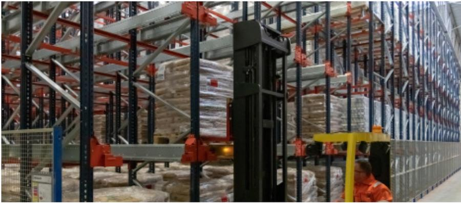
Workers deposit the Pallet Shuttle in the corresponding channel. Soon afterward, they insert the goods in the channel's first position and the motorised shuttle takes it directly up to the first open location it finds inside the channel. Operators use a tablet with a WiFi connection to interact with the shuttles and organise the introduction and extraction of the pallets. And, seeing that operators do not need to enter the lanes to handle the goods, this reduces potential damage to the racks.
