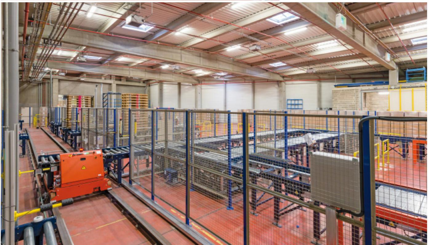
The conveyor circuit also incorporates a full pallet stacker, which can lift the pallets to place them on slave pallets, and a station where empty pallets are stacked and unstacked.
