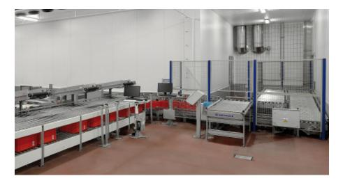
The products are previously placed in plastic boxes of the eurobox type, measuring 600 x 400 x 300 mm, forming a transport and storage unit
