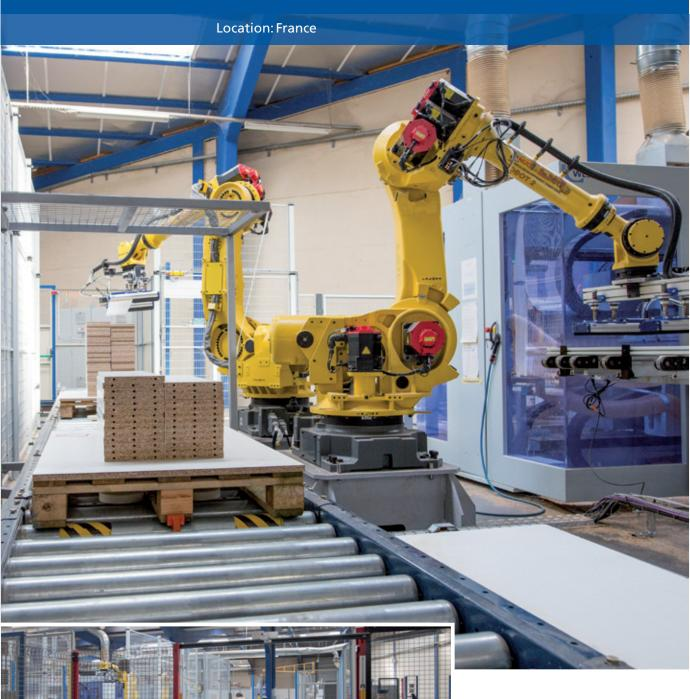
Mecalux has installed a high-tech conveyor circuit in the production centre of Euréquip, a French furniture maker. It is arranged to move goods to and from the various processes that mould the wood panels used to manufacture furniture. This transport system provides speedy relocation of goods to the positions needed for each operation.
