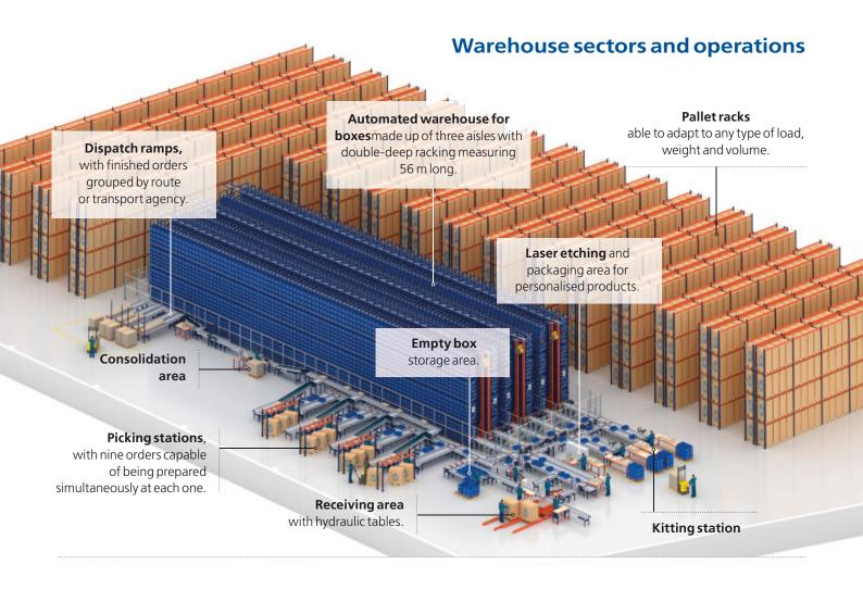
The automated warehouse for boxes, meanwhile, can store 80% of SAM Outillage's SKUs. This system was chosen primarily to stock items more densely, as it is able to hold a large number of products in a limited space. The installation is made up of three aisles with 40-metre-long double-deep racking on each side that can accommodate up to 20,000 boxes measuring 400 x 600 mm with three different heights.
