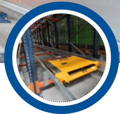
The goods are inserted on one side of the racking and removed on the other. Thus, they are stored according to the FIFO (first in, first out) method, ensuring that the company distributes products with an earlier expiry date before others.
