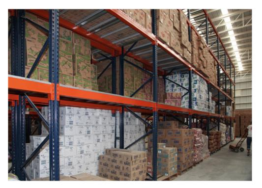
Mixing and matching single- and double-depth racks mean SKUs can be organised according to their features and demand level. In the words of Álvarez Mendoza, "Double-deep pallet racks were chosen because they entail a space savings that requires fewer aisles to access the loads. Plus, this solution ensures maximum storage capacity."
