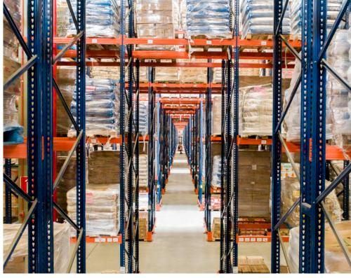
almost the entire surface area and facilitate goods management. On a normal working day, the operators walk through the storage aisles introducing and removing pallets from their corresponding locations using reach trucks.
