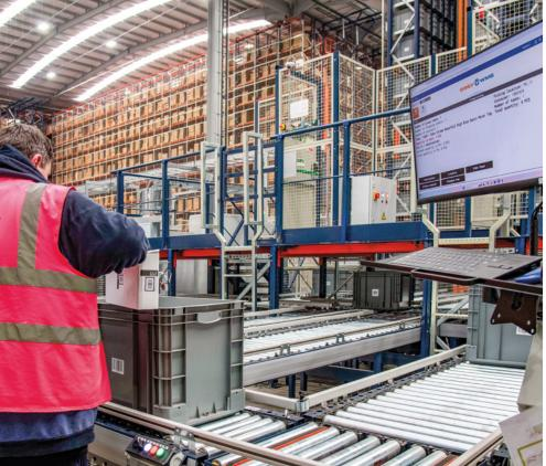
To speed up order fulfilment, conveyors automatically transport pallets and totes containing all types of bathroom items and accessories to the pick stations
