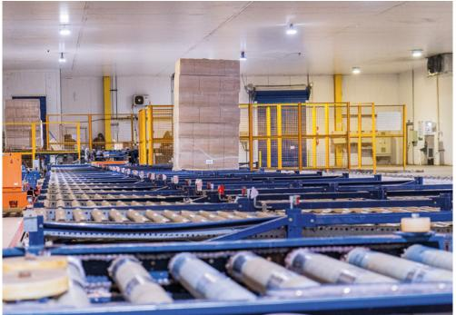
Inside, the Automated Pallet Shuttle system stores and retrieves goods autonomously, speeding up pallet putaway and dispatch operations. Conveyors automatically connect the automated warehouses with the production and shipping areas.
