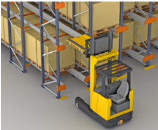
STEP 1 A forklift places a Pallet Shuttle on the level where the goods will be stored.
