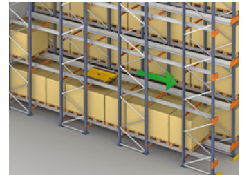
STEP 4 The shuttle returns to the lane entrance to repeat the procedure with the next pallet, continuing successively until the lane is full. Once the last location is filled, the shuttle is extracted, ready to work on another level.
