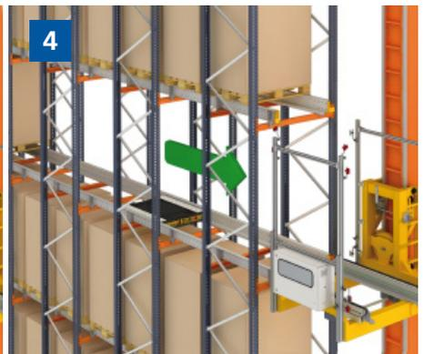
4. The stacker crane waits for the Pallet Shuttle to finish and move automatically back onto the cradle.
