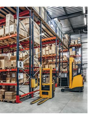
with Movirack mobile pallet racks to hold an additional 1,120 pallets.
