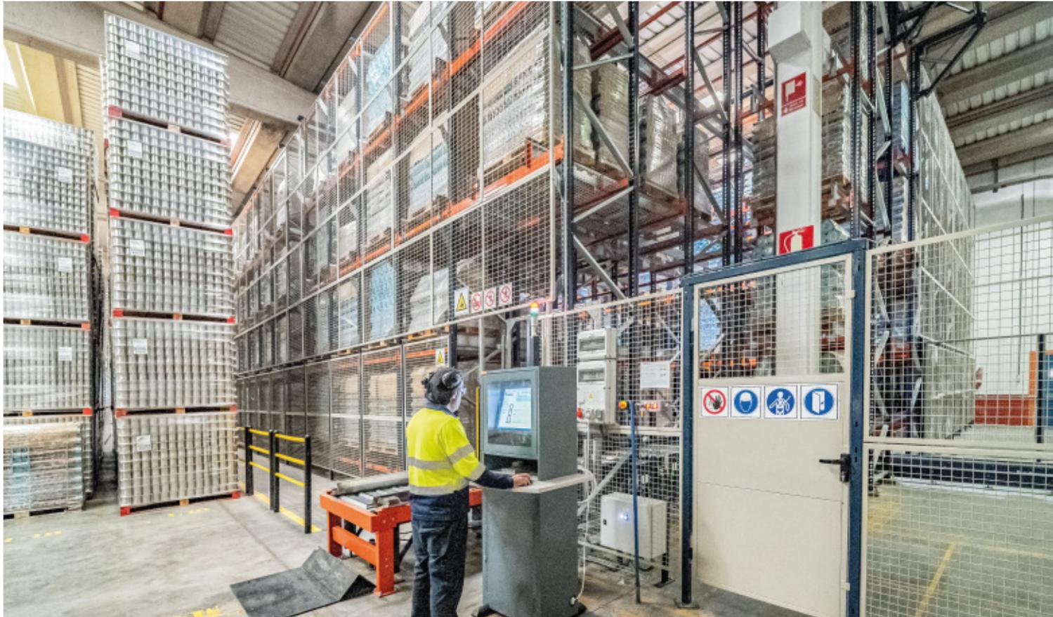
er crane. This high-density automated storage and retrieval system (AS/RS) has boosted efficiency in the Envases Group facility. In addition to making the most of its floor space to expand storage capacity, the company has leveraged automation to streamline and maintain stricter control over incoming and outgoing goods.
