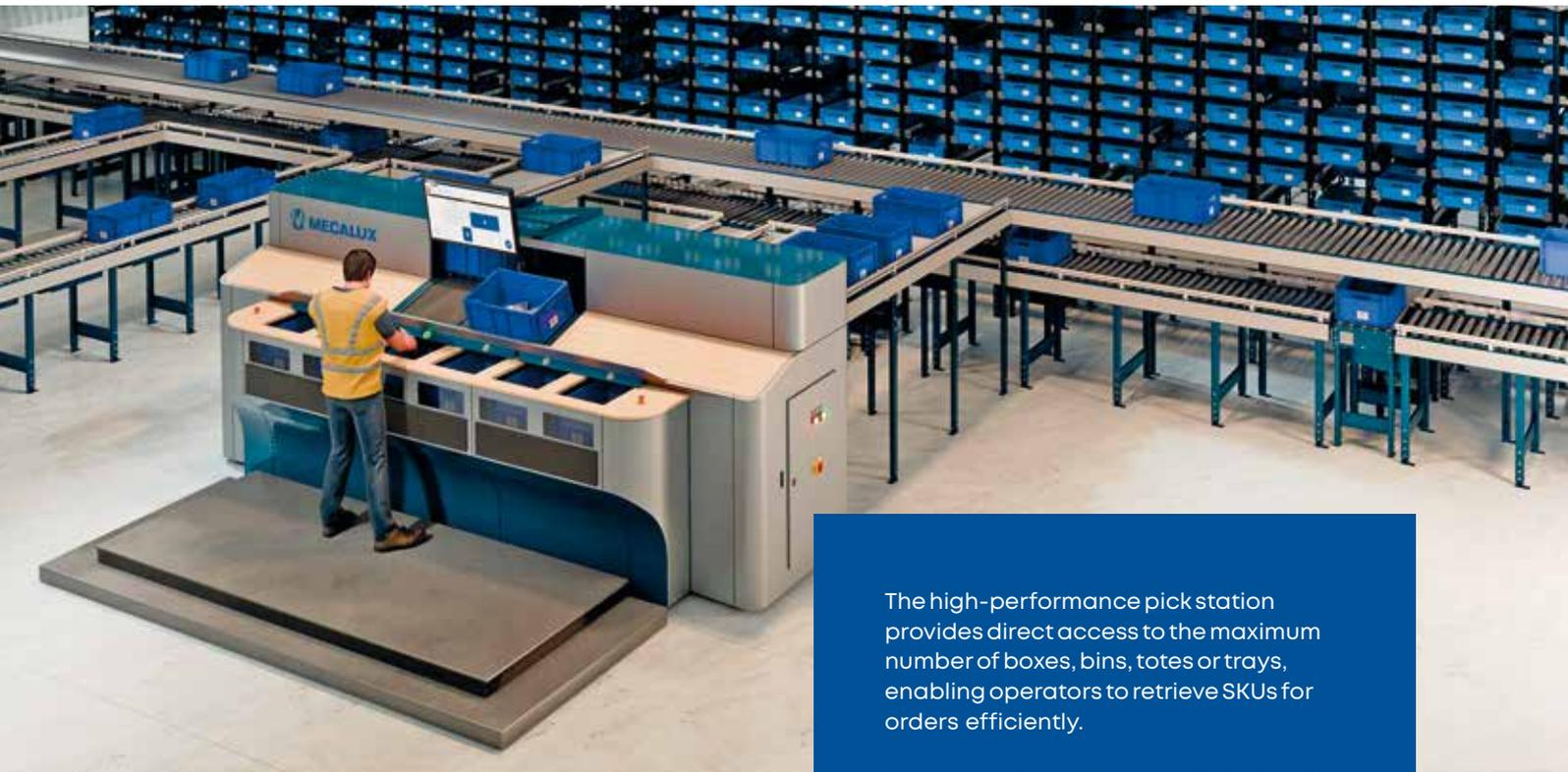
The high-performance pick station provides direct access to the maximum number of boxes, bins, totes or trays, enabling operators to retrieve SKUs for orders efficiently.
