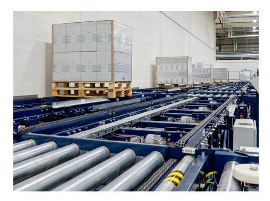
streamline this work. Orders are prepared according to the product-to-person principle, which reduces operator travel and increases speed.
