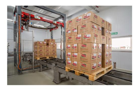
Mecalux proposed installing the automatic version of the Pallet Shuttle system with stacker crane because it combines all the advantages of high-density storage and automation. This solution is the result of merging the storage capacity of high-density systems with the reduction in the time spent on each operation, typical of automated systems.
