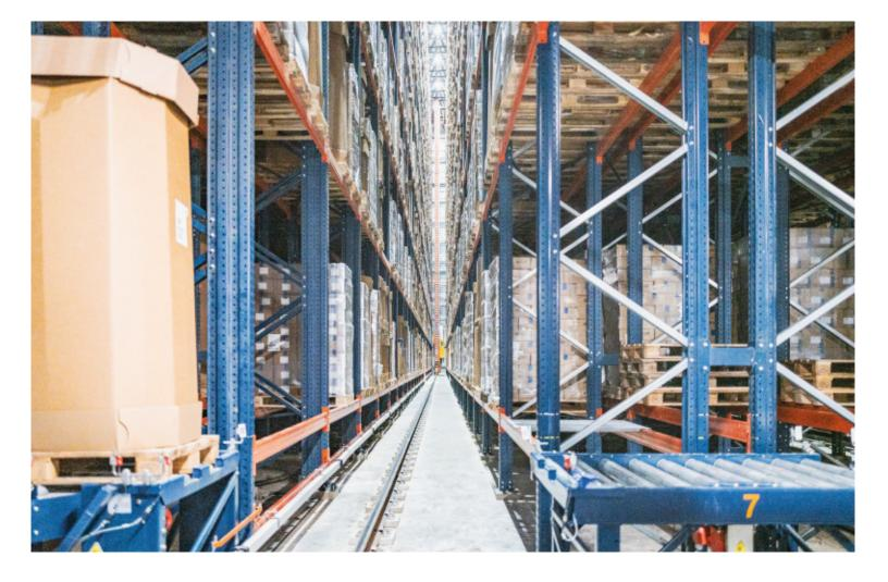
mising the facility's floor space, this high-density storage and retrieval system (AS/RS) for 7,000 pallets has cut energy consumption; making better use of space reduces the volume of air to be cooled. Now, Saar has tripled its production pace, yielding up to 24,000 tonnes of deep-frozen vegetables annually.
