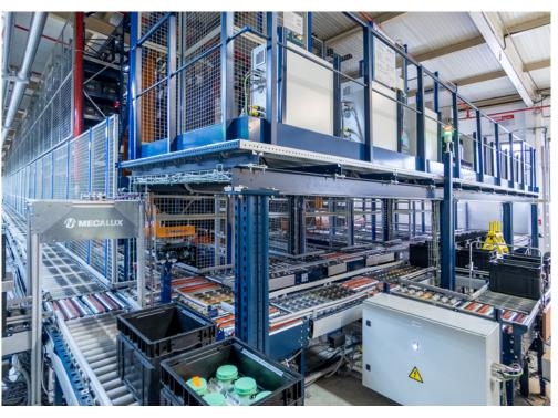
The AS/RS comprises three aisles with double-deep racking on each side. In this small space (the racks stand 4 m high by 28 m long), Schaeffler can store up to 490 different SKUs in 5,184 boxes measuring 396 x 297 mm with a maximum unit weight of 65 kg.
