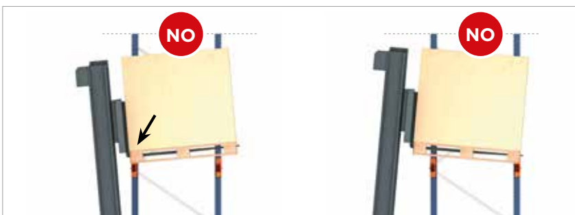
Figure 9. Beam overloading from not lowering a pallet horizontally .
