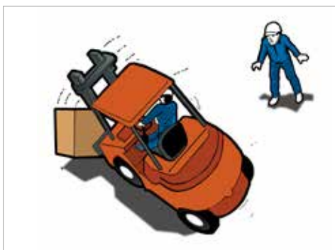
Figure 8. Losing control of the forklift.
