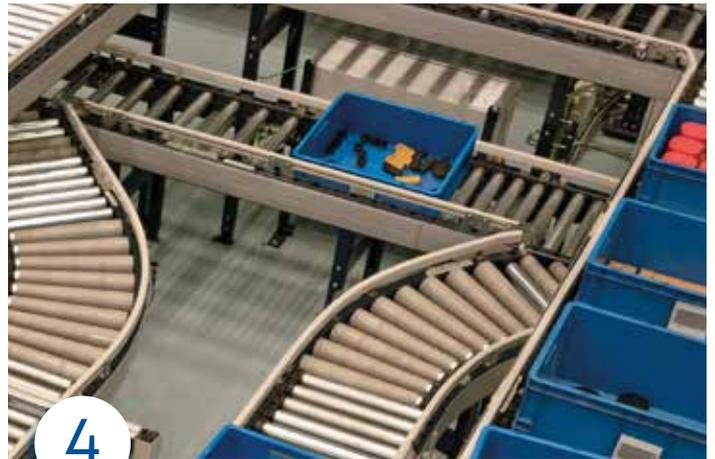
**Picked order.** Once picking has finished, conveyors transport the tote containing the order to another area in the facility (consolidation, dispatch, etc.).
