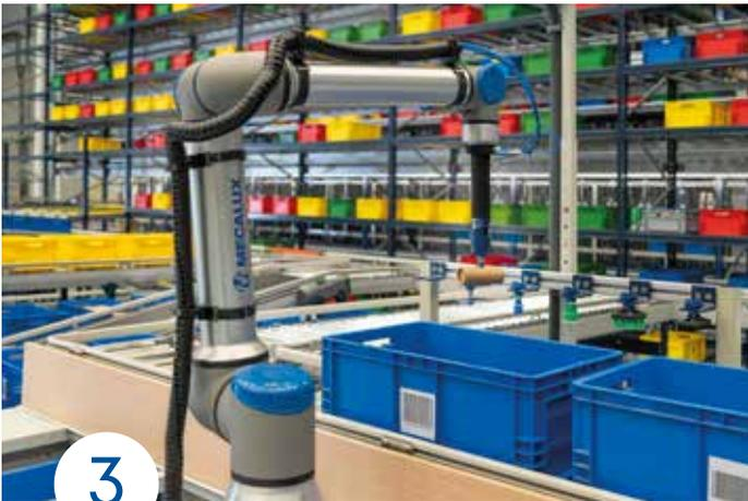
**Product picking and placing.** Using the data provided by the Siemens vision software, the robotic arm picks the selected product and places it in the corresponding order tote.
