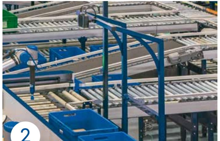
**Product identification.** The vision system's camera takes a picture of the inside of the storage tote containing the SKUs. Then, the vision software analyses the picture captured to identify the silhouette of the product to be picked and determine the best way to do so.
