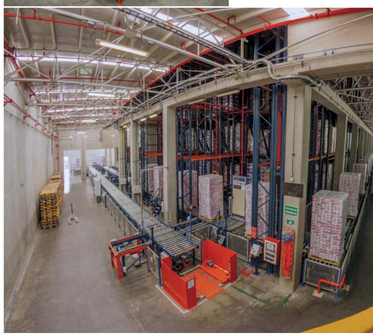
The recirculating conveyor circuit (double circuit) allows the management of inputs coming from production and from outside, as well as direct dispatches of palletised goods from the warehouse
