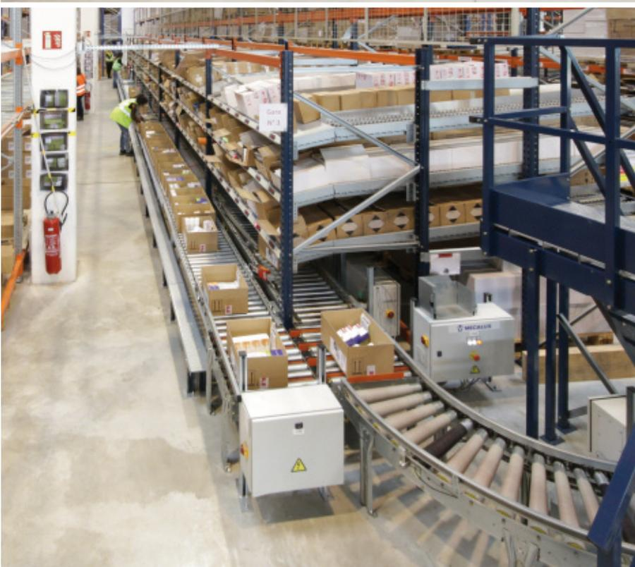
**Mecalux automated a portion of the warehouse that AS Healthcare owns close to Paris in order to guarantee efficient picking, save on logistics costs and reduce the margin of errors during handling. The solution consisted of live pallet racking with the pick-to-light system and a conveyor circuit with rollers that joined the prep zone to the sorting and consolidation areas.**
